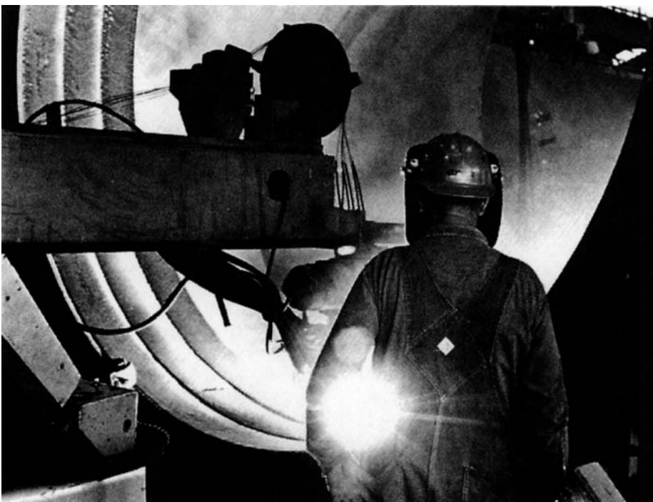
Process reactors in a petroleum refinery can either be solid stainless steel (above), clad, or protected with a weld overlay (below), such as might be used in an HDS reactor. Photographs: Wyatt Industries, Inc.
